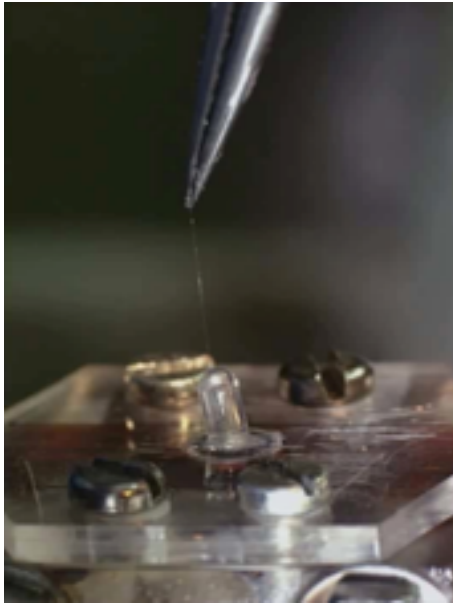
Mulberry silk is converted to spider silk using only pressure and moisture controls just like the spider does. Photo courtesy of Oxford Biomaterials (UK).
